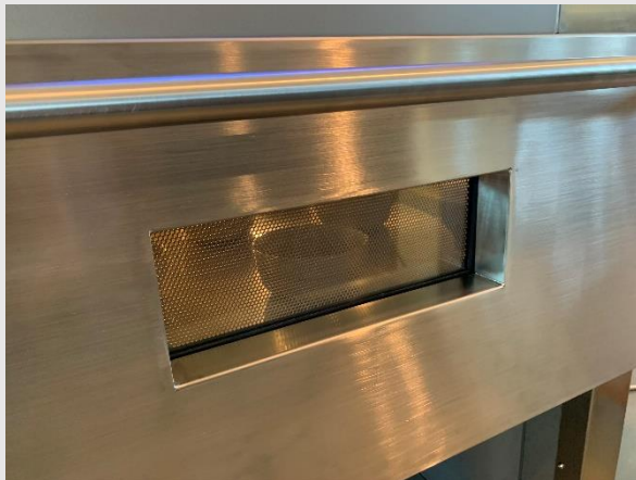
Frame with very powerful light inside the chamber to check the treatment process.
