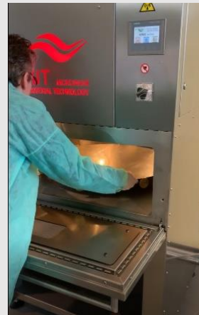
Ordinary cleaning can be carried out safely by a single operator. The room can be clean at every corner. The turning plate can be removed and washed separately.
